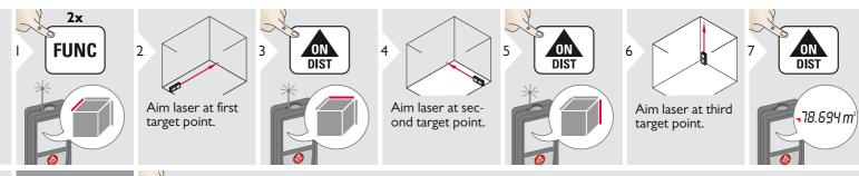
The result is shown in the main line and the measured value above.
