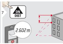
The result is shown in the main line and the measured distance above.
