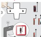
Distance is measured from the rear of the device (standard setting).
