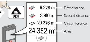
The result is shown in the main line and the measured value above.
