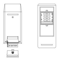
• HI 93501, HI 95502, HI 93503 and HI 935007: the batteries are accessed by separating the front and the back halves of the meter. Unscrew the 4 screws on the back of the meter and carefully replace the three 1.5V AA alkaline batteries located in the battery compartment, while paying attention to their polarity. Reattach the back making sure that the gasket is in place and tighten the 4 screws to ensure a watertight seal.
