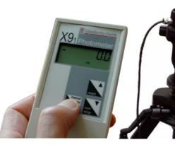
diagnostics for example. For this reason current DIN and EN regulations specify that light meters must have a maximum permissible error  $f_{tot}$  of ±10%. According to DIN-5032 Part 7 these are regarded as DIN class B instruments. This quality designation is necessary because class C instruments - incidentally many photometers on the market are not certified at all - that are used to measure different types of light sources such as standard illuminant A incandescent lamps,
