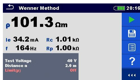
Figure 11.39: Example of Wenner method measurement result
