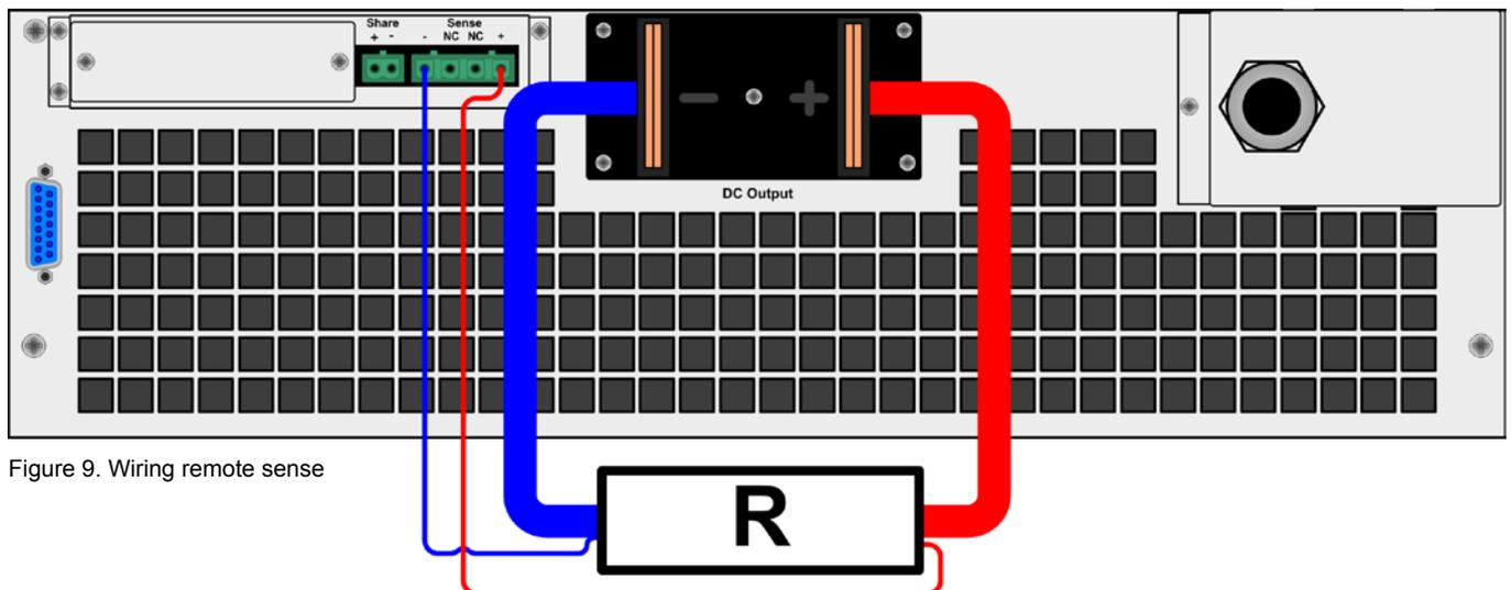
Figure 9. Wiring remote sense
