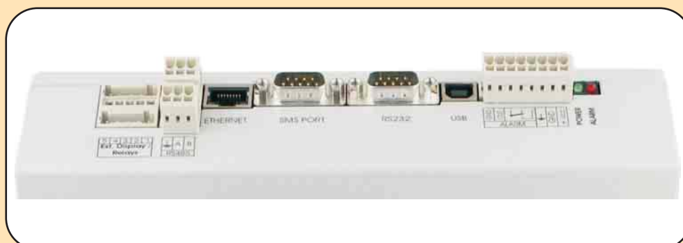
Power and communication connectors, alarm outputs
