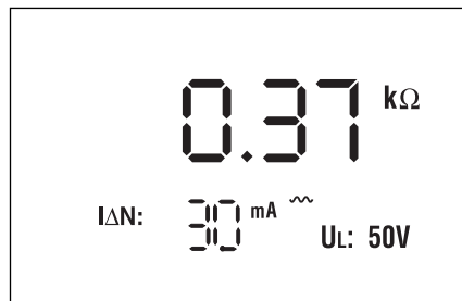
Display at earth resistance
